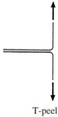
Figure 5 – A diagram of a T-peel test (Material-Welding, 2022)
